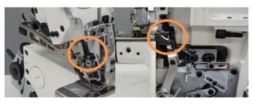
DLC needle bar and upper looper holder preventing oil leakage
