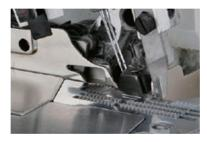
**Side chain cutter(VTC)** is only available with cylinder type overlock
