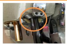
**Needle bar oil return system** Protects the fabric from the oil stain
