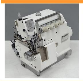
2 needles 4 threads overlock with 148mm circumference cylinder.
